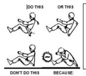
Seat Belts are supposed to restrain the up and down movement and the shoulder harness prevents forward movement, hence the recommended mounting locations.
